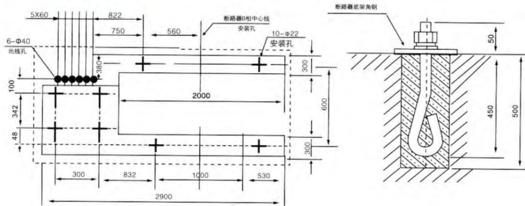
LW8A-40.5(中置式)外形安装尺寸(middle type) outline mounting size
